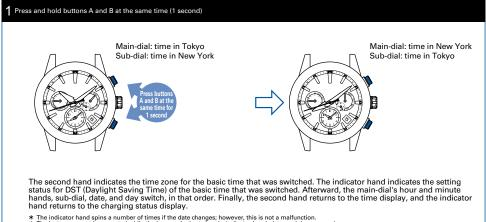
\* The buttons cannot be operated while the hour and minute hands, indicator hand, date, and day are moving.
